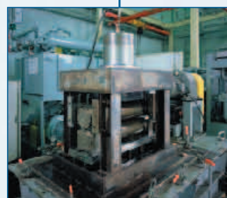
Tester for bearings used in guide rolls of continuous casting machines
